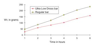
Results are based on an "in-house" experiment using an aerated 2000 gram solder pot at 260℃ (500年).
